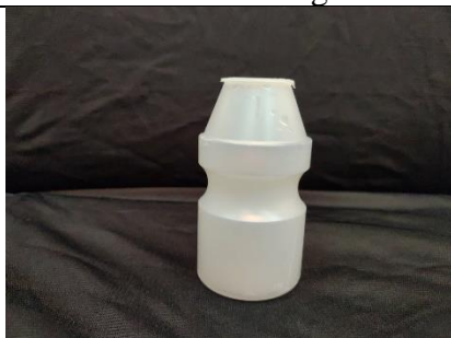
Figure 9.4.2.-3 Image of small bottle, approximately 8.5 cm in height, with a mouth 4.5cm in diameter, weight 7 grams.
